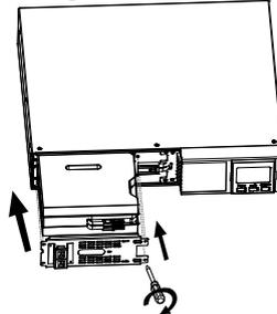
After replacing the batteries, put the battery box back to original location and screw it tightly.
