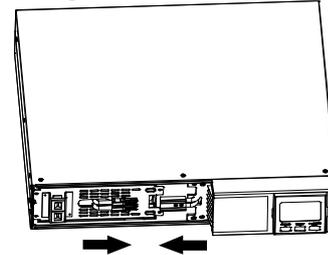
Re-connect the battery wires.
