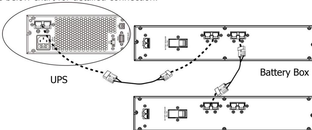
**NOTE:** Maximum connected external battery boxes up to 4 units.
