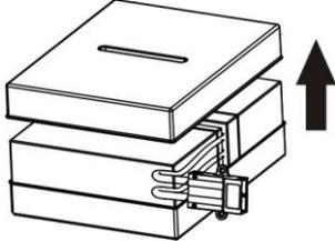
Remove the top cover of battery box and replace the inside batteries.
