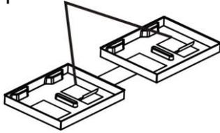
Step 3: Put assembled battery packs on one side of plastic shells and insert one more defect battery on the space.
