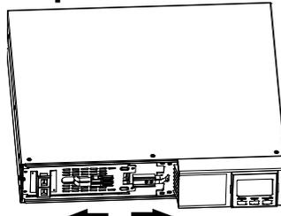
Disconnect battery wires.
