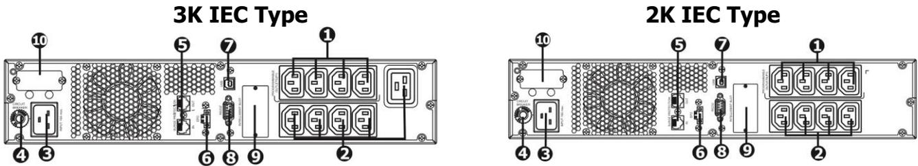
1. Programmable outlets: connect to non-critical loads.
